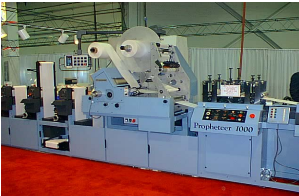
The Tamarack P500 in-line on a Propheteer press, applying transfer tape to produce integral labels.
